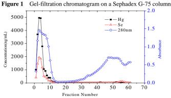
The supernatant extracted from the liver powder by alkaline protease in the presence of 1%SDS was subjected to the column ( $1.2 \times 60$  cm). Eluent: 0.1 mol/L NH<sub>4</sub>Ac-NH<sub>3</sub> (pH 9)
