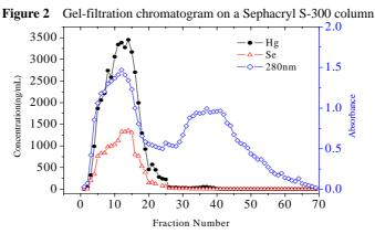
The fractions of void volume on Sephadex G-75 were lyophilized and the mixture of it reacted with DDT and DDTC was subjected to the column  $(1.2 \times 60 \text{ cm})$ . Eluent:  $0.1 \text{ mol/L NH}_4\text{Ac-NH}_3$  (pH 9)
